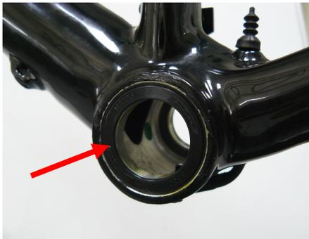
5. Install the Bearing Shield ④ on the right Bearing, with flange (machined grooves on alloy covers) toward bearing.
