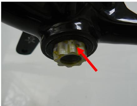
6. Insert the right crank arm and spindle through the both BB30 bearings. Position non-drive side bearing shield ④ over left bearings with flange inward, toward the bearings. (as shown in photo)
