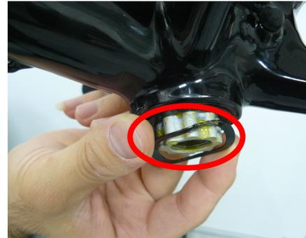
7. Position the wave spring washer ⑤ on the spindle on non-drive side.
