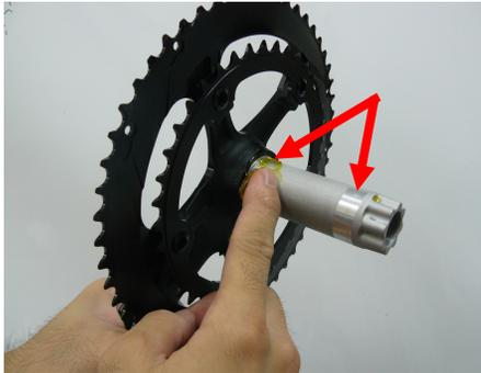
4. Apply grease to the machined surfaces of the spindle that will contact the bearings after crank installation (as shown in photo).
